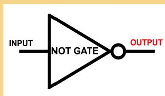
NOT gates can be used to turn an output device off when a switch is turned on e.g. emergency stop button.
