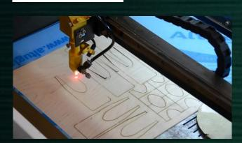
Laser cutting involves a beam of light that vaporises through a piece of material to cut a shape to the desired shape.
