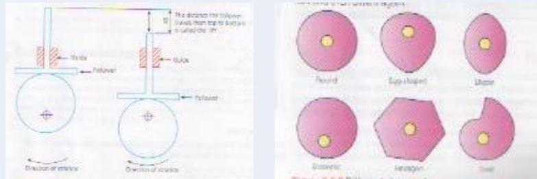
The pattern of movement is determined by the design / shape of the cam, i.e. if the cam is round with the shaft in the centre the follower will remain stationary, however if the cam is round but the shaft is off centre then the follower will continually rise and fall.
